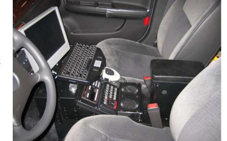
C-TM-IMP-1 installed w/ console, computer mounts and accessories. (Sold separately)
